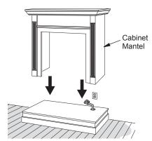
Figure 10 - Installing Cabinet Mantel
